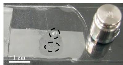
Figure 3. Picture of a G1657 adhesive design after testing with air film trapped. The top circle shows a large air bubble that coalesced after partial wetting occurred around the areas under test (shown approximately with the ellipse). Partial wetting occurred in an area approximately 1 cm in diameter.
